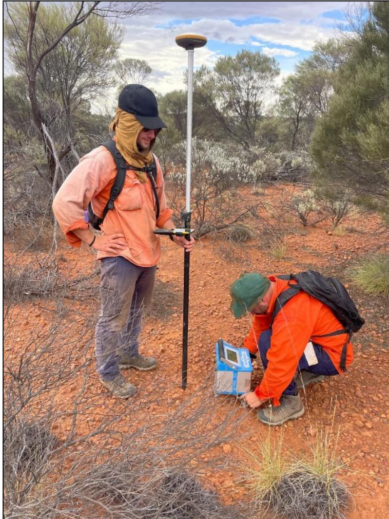
Figure 1: Atlas Geophysics consultants collecting high resolution ground gravity data across Dusk 'til Dawn
