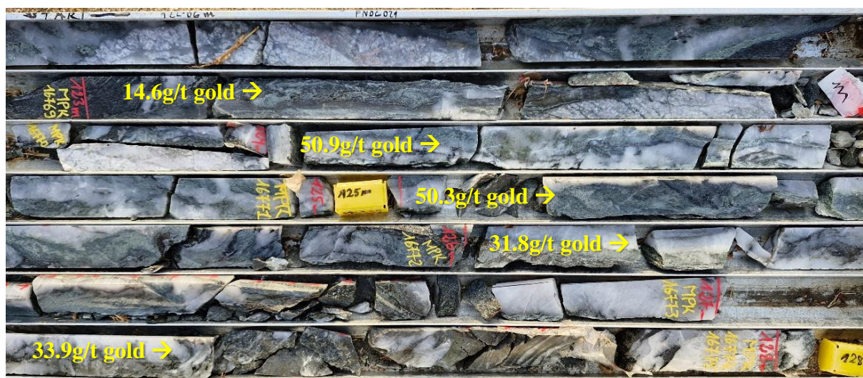
Figure 2 | FNDC021 Interval from 122.06m to 128.05m drill depth in felsic intrusion with quartz veining and sulphide mineralisation, with sample interval from 122m to 128m averaging 41.2g/t gold
