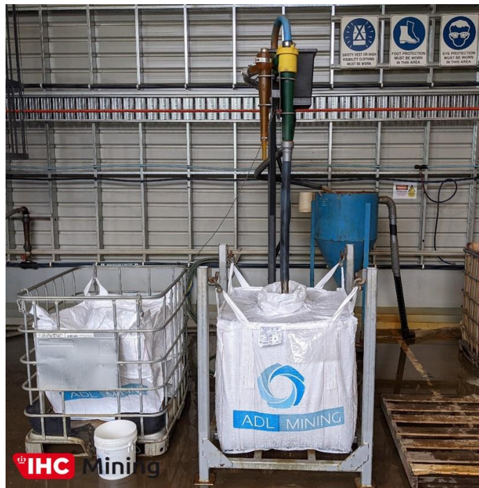
Plate 4 – Slimes removal (material <45µm)
