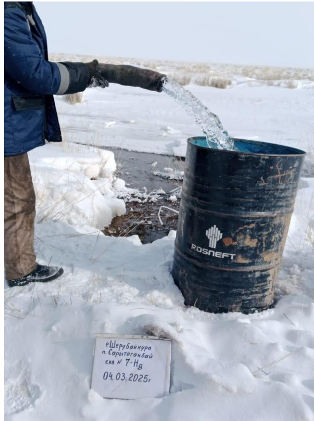
Figure 3 – Pump testing of the HG7 water bore.
