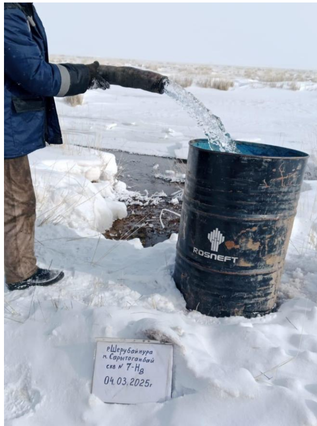
Figure 3 – Pump testing of the HG7 water bore.
