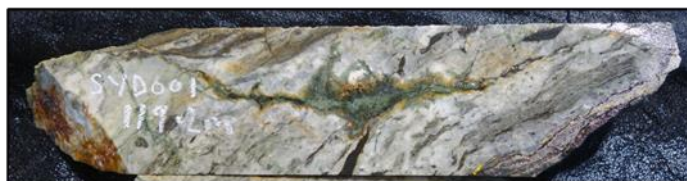
Figure 8 – RC Chip photos and core photos with assay data of the newly defined carbonate hosted high grade gold intersections at Sunraysia (information from historical drilling, refer to Appendix 1 for more information)
