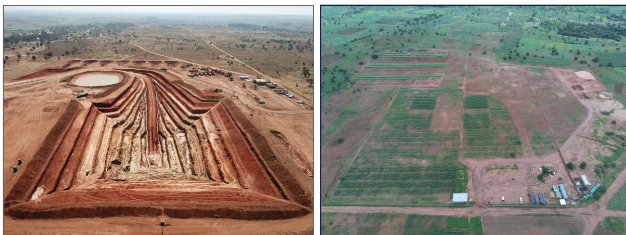
Figure 2: Pilot Phase test pit during mining trials (left) and subsequently backfilled and rehabilitated (right)
