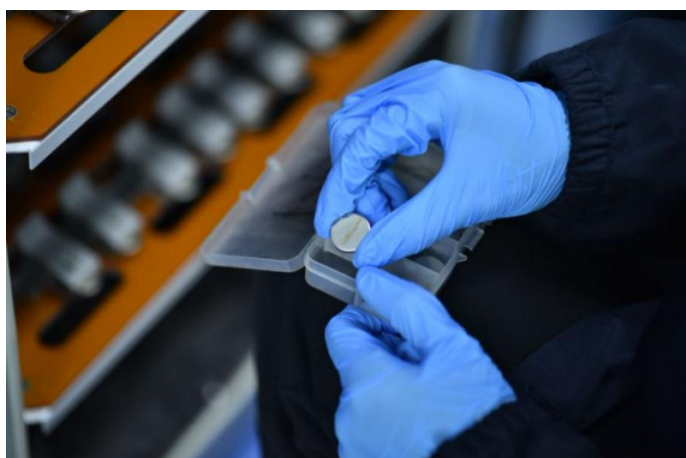
Image 1: Button batteries made with Firebird LMFP, Note: Battery industry standard to conduct battery testing on button batteries
