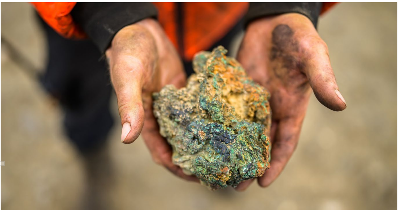
Figure 7: Copper gossan from the Hailstorm Prospect. This is massive chalcocite (copper sulphide) and returned a laboratory assay grade of >50% Cu, 61g/t Ag (Sample Y007193, 50% Cu is the upper limit of the assay technique used).
