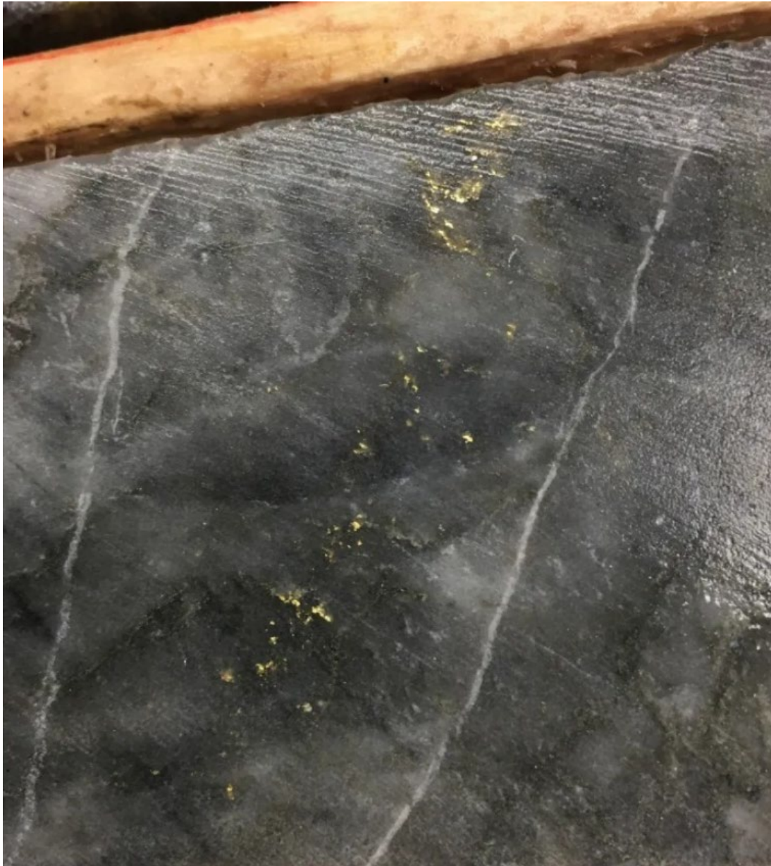
Figure 2 Photo of core from drillhole BO-21-08 at the Paquin East prospect showing Visible Gold within characteristic blue-grey quartz (184.5m). The one metre interval 184-185m assayed 1m@ 129.25g/t Au. This was within 9m @ 16.96g/t Au from 178.5m 6 .
