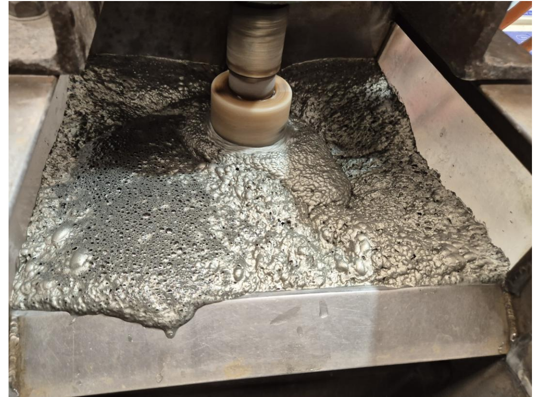
Cleaner flotation – increases gold grade and reduces concentrate mass
