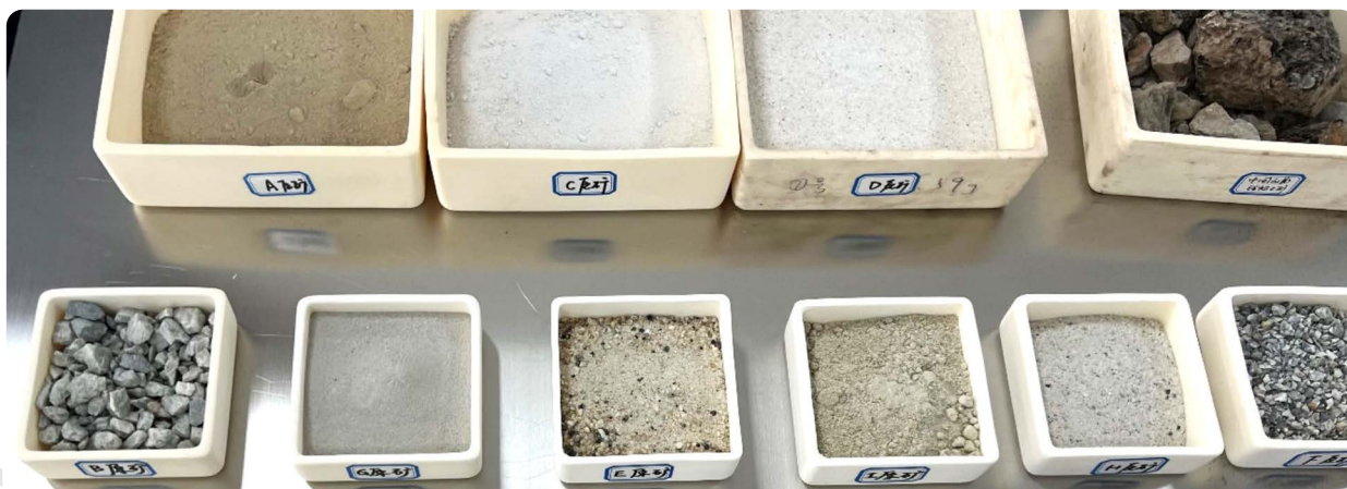
Figure 13: Various Spodumene Concentrates from around the world showing various particle sizing and grades
