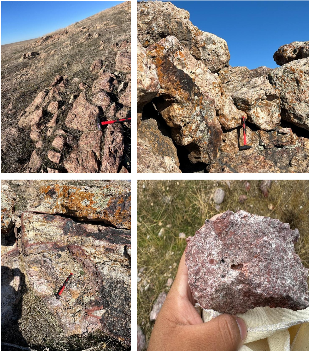
Figure 3 - Hydrothermal alteration at Zholbars prospect, December 2024.
