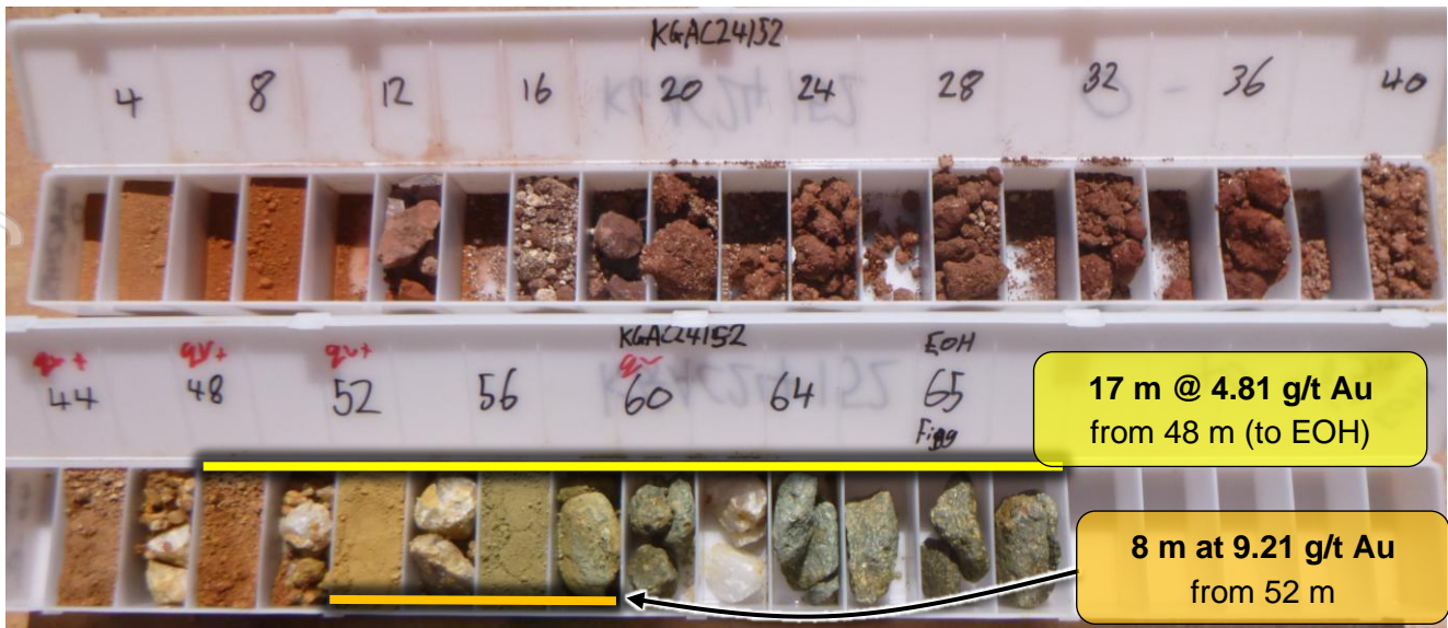
Figure 3 – Archived rock chips and spoil from drill hole KGAC24152, displaying gold grades downhole. Here the supergene gold blanket coincides with oxidation of the profile (transition from greenish fresher intermediate to mafic volcanic to subvolcanic rocks at base to ochre and red weathered rocks (and red transported cover) higher in the profile. In this hole, the supergene blanket interacts with primary gold mineralisation, which is likely hosted (at least partially) by quartz veining (white fragments).
