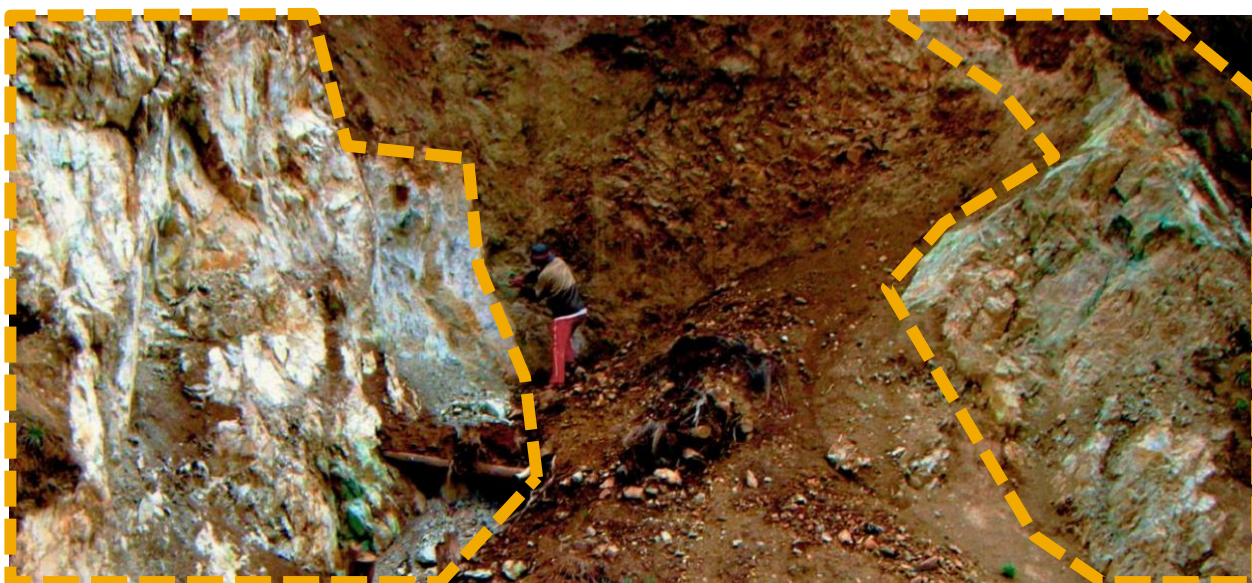
Figure 4: Historic sampling of felsic diorite porphyry outcrop with copper bearing malachite, at Venatica West showing cooling joints in contact with mineralised Breccia which returned 4.6% copper in sample 2253. Man is facing rock-chip sample site, orange outline shows outcropping sections of the porphyry which continues out of image.
