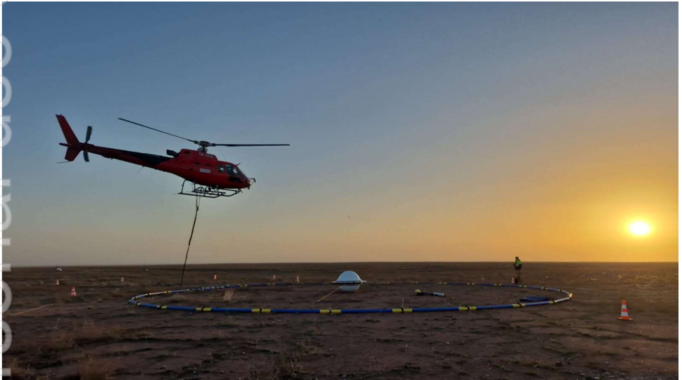
Figure 2 – Survey helicopter and Electromagnetic loop during survey testing
