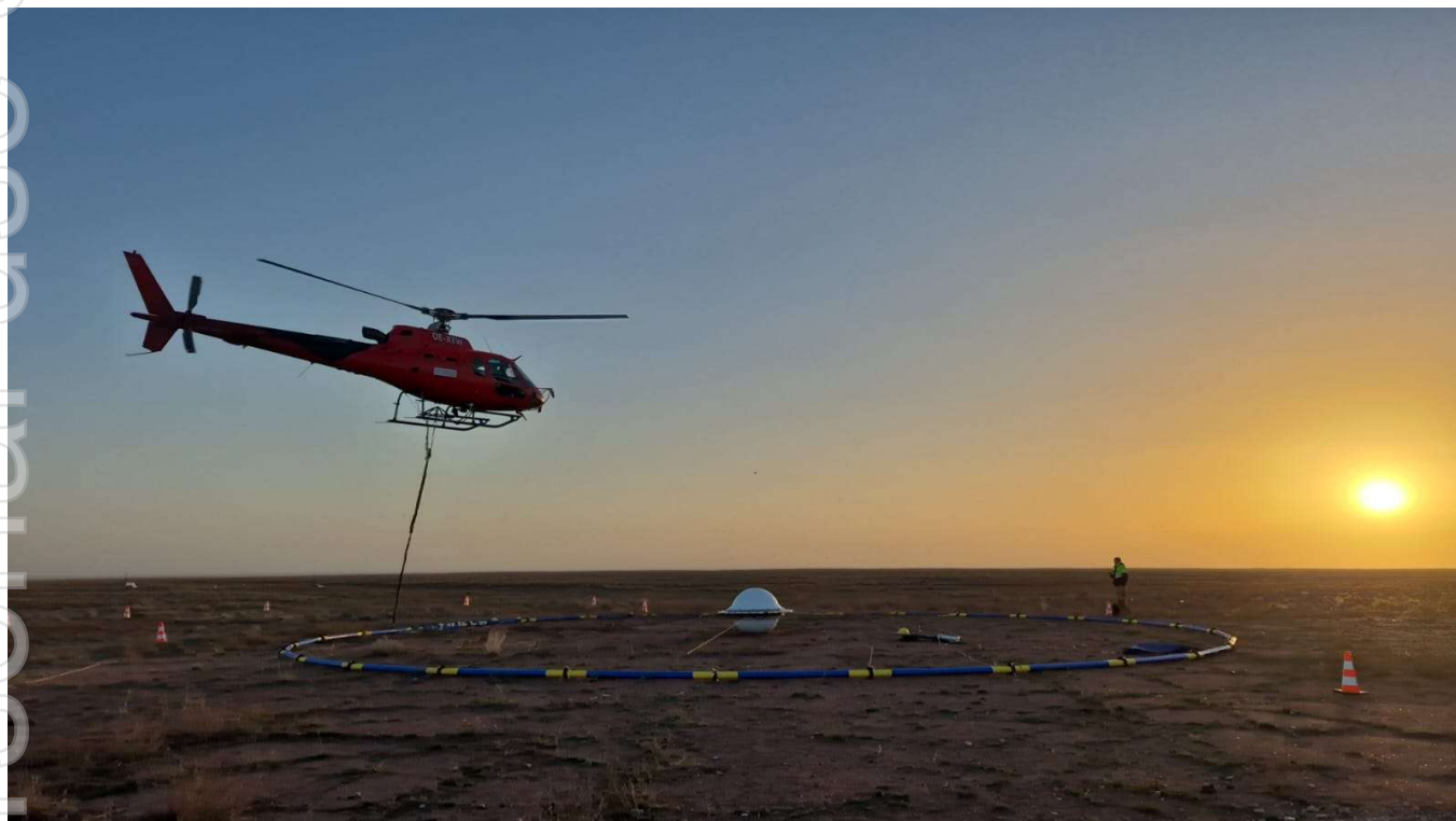
Figure 2 – Survey helicopter and Electromagnetic loop during survey testing
