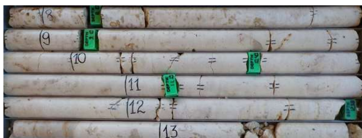
Fig 1 - Soalara Limestone - High purity @ 97% Calcium Carbonate
