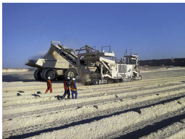
Fig 2 – Example Surface Miner – Limestone row cutting
