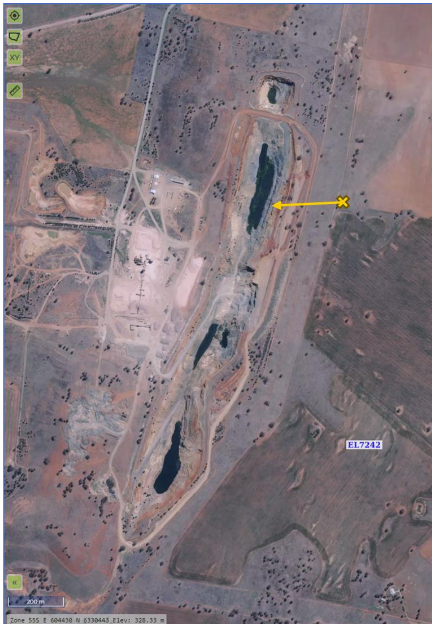
Figure 3 – Satellite image of the historic London-Victoria pit showing AEIDD001's collar location and drillhole trace.
