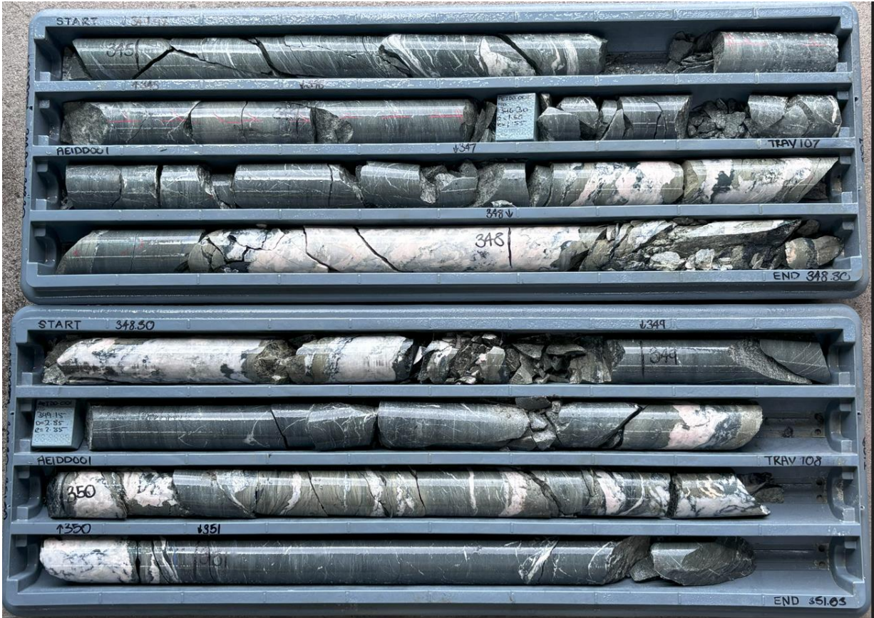
Figure 4 – Photo of core trays 107 and 108 from DDH AEIDD001 (344.97-351.63m) showing most of the 12m-thick zone of quartz-carbonate veining and shearing in sericite-pyrite altered andesitic volcanoclastic rock intersected 339 to 351m downhole, which is thought to be the down-dip extension of the London-Victoria deposit. Core tray length is 1m.
