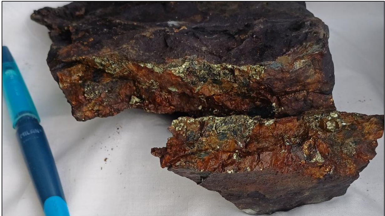
Plate 2: Chalcopyrite-quartz vein hosted in paragneiss. 4.4% Cu, 0.01% Ni, 1.8 g/t Au, 0.50 g/t Pd, 0.06 g/t Pt. Virdnechokka area, sample 14508.
