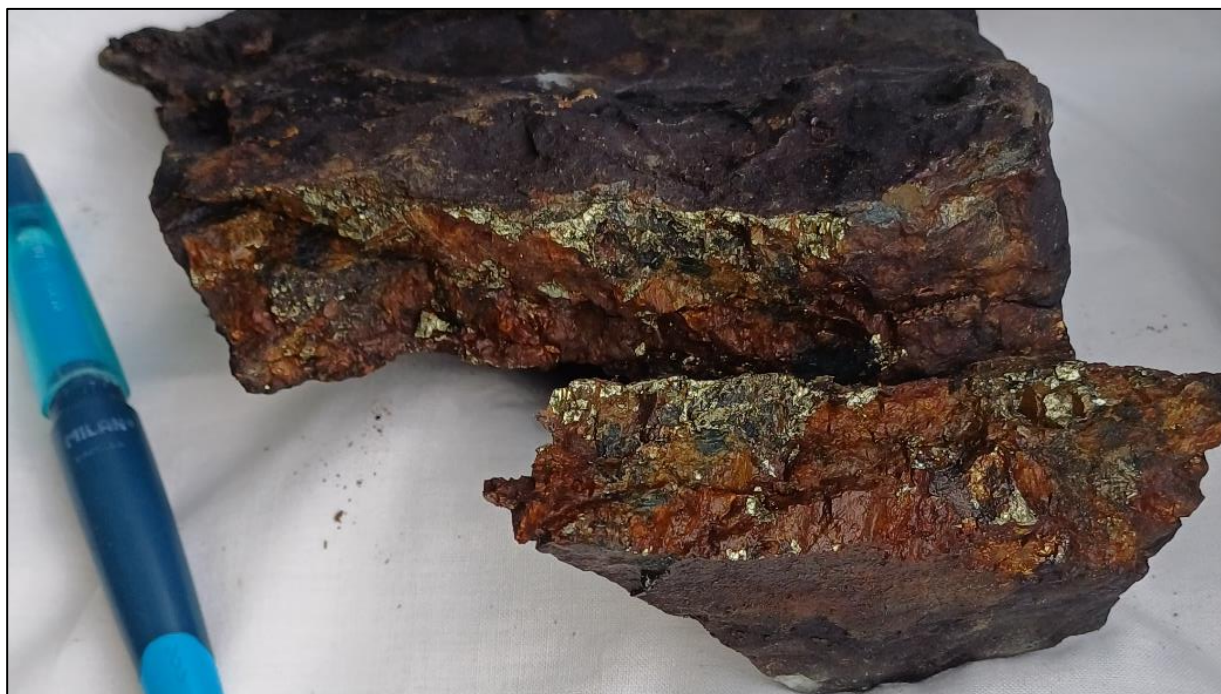
Plate 2: Chalcopyrite-quartz vein hosted in paragneiss. 4.4% Cu, 0.01% Ni, 1.8 g/t Au, 0.50 g/t Pd, 0.06 g/t Pt. Virdnechokka area, sample 14508.
