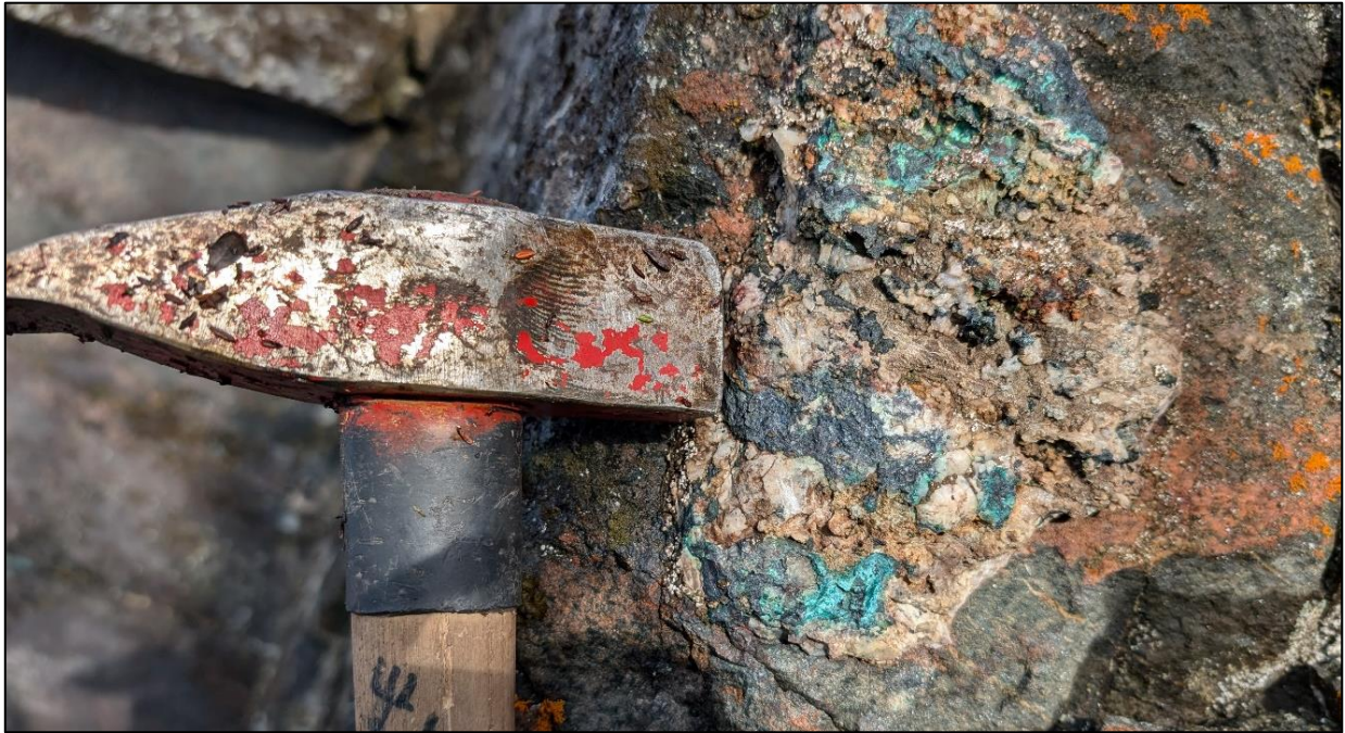
Plate 1: Chalcocite-bornite-quartz vein hosted in amphibolite. 29.7% Cu, 0.01% Ni, 1.1 g/t Au, 53 g/t Ag, 0.54 g/t Pd, 0.02 g/t Pt. Porsanger area, sample 14398.
