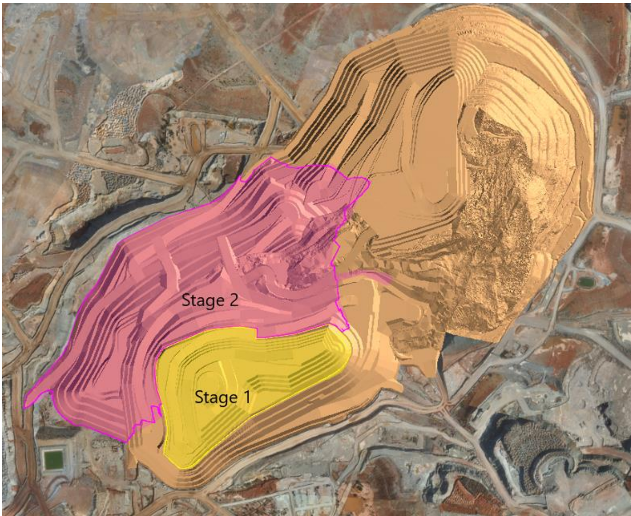
Figure 3: King of the Hills open pit highlighting stage 1 & 2 design in the southern section of the LOM Ore Reserve pit shell
