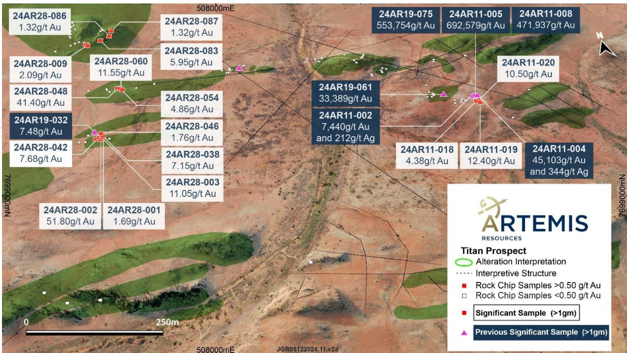
Figure 4. Satellite image of the Titan Prospect showing location of high-grade surface samples from quartz/ironstone veins and gossanous chert outcrops around the interpreted gravity-low feature.
