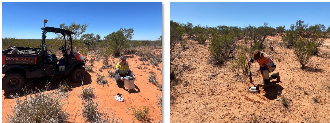
Figure 3. Ground gravity and ANT surveying over the Cuttaburra area. Figure 4. ANT geode placed into the ground to take passive seismic readings continuously over seven days of deployment.
