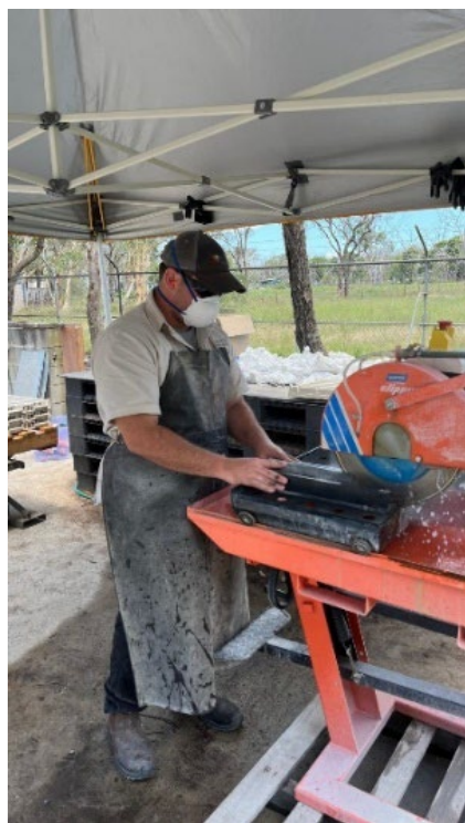
Figure 1: Field team sampling historical drill core. Figure 2: CUTBD02, 419.8m – Unsampled banded arsenopyrite (grey) in quartz vein (see Appendix 1 & 2, Drill Log Summaries) v .
