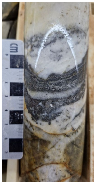
Figure 1: Field team sampling historical drill core. Figure 2: CUTBD02, 419.8m – Unsampled banded arsenopyrite (grey) in quartz vein (see Appendix 1 & 2, Drill Log Summaries) v .
