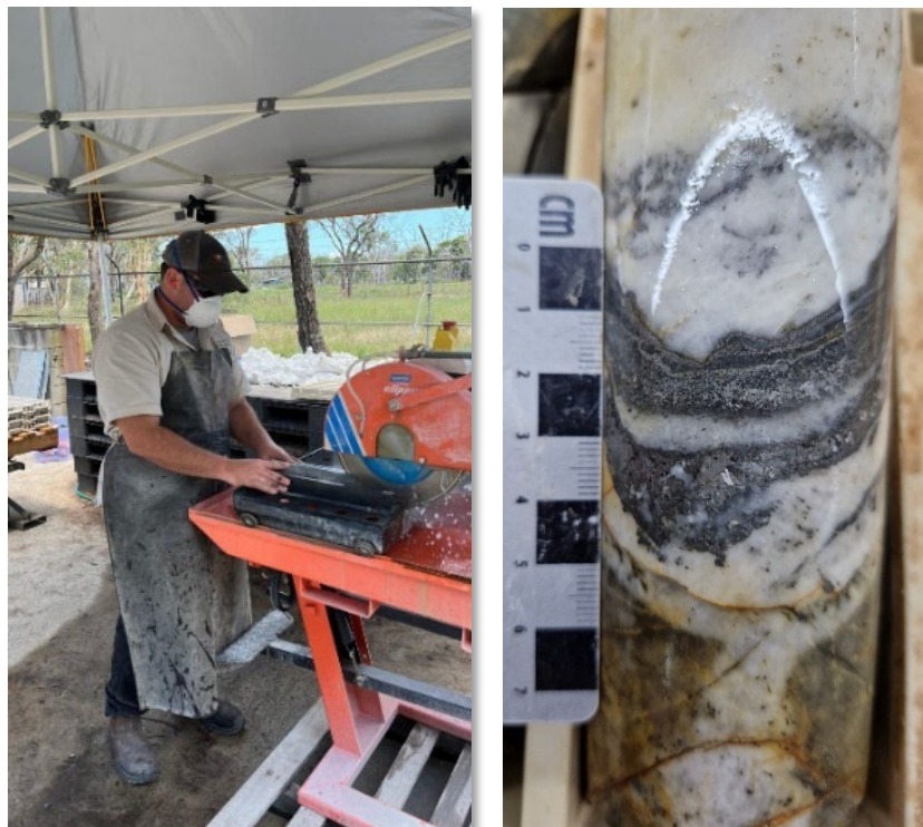
Figure 1: Field team sampling historical drill core. Figure 2: CUTBD02, 419.8m – Unsampled banded arsenopyrite (grey) in quartz vein (see Appendix 1 & 2, Drill Log Summaries) v .
