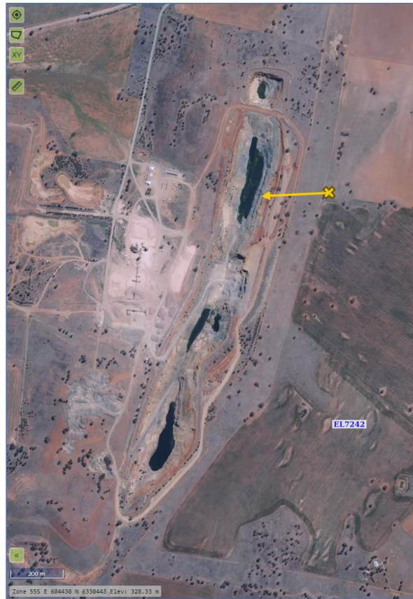
Figure 5: Satellite image of the historic London-Victoria pit showing AEIDD001's collar location and drillhole trace.
