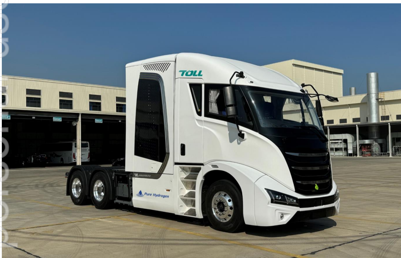
An image of the Taurus 70t HFC prime mover to be supplied to TOLL Transport
