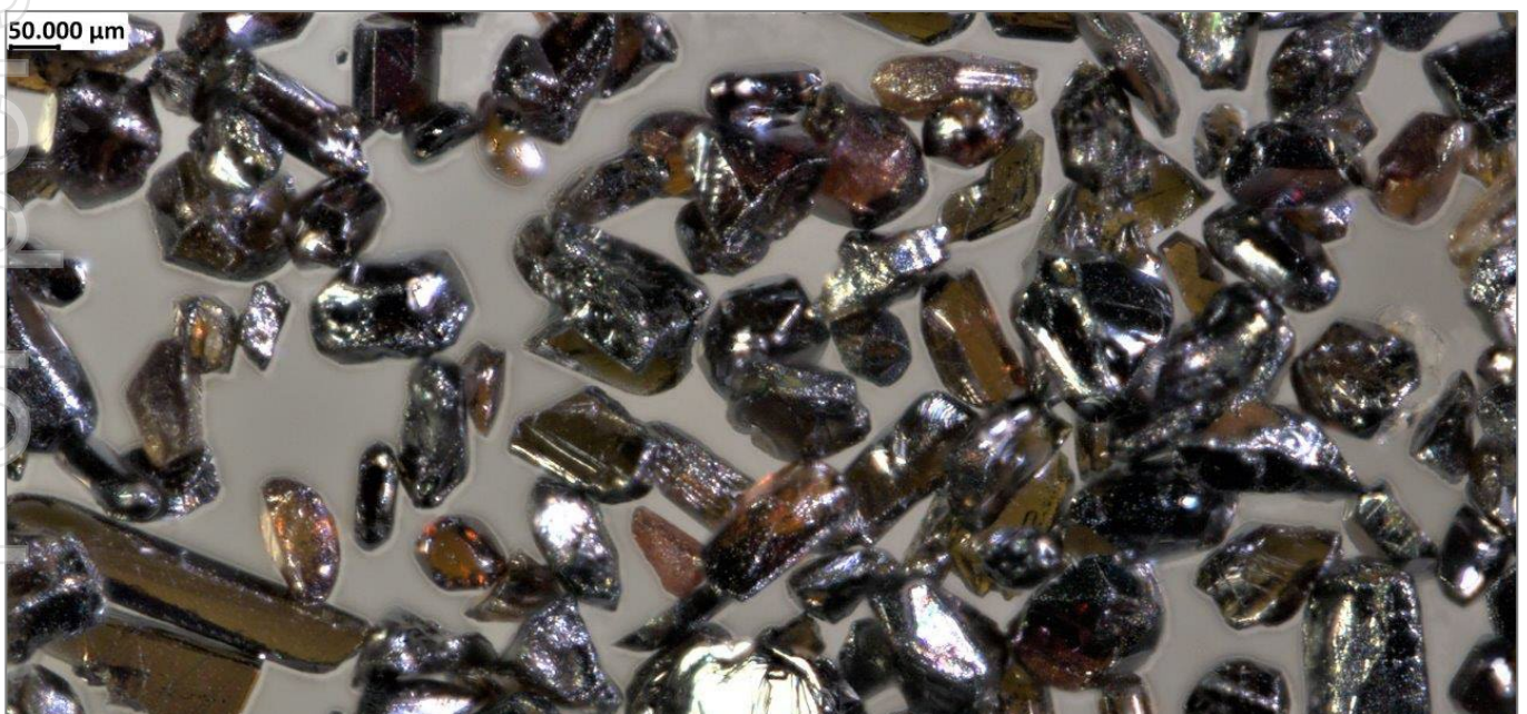
Figure 17: Photomicrograph of high-purity rutile product
