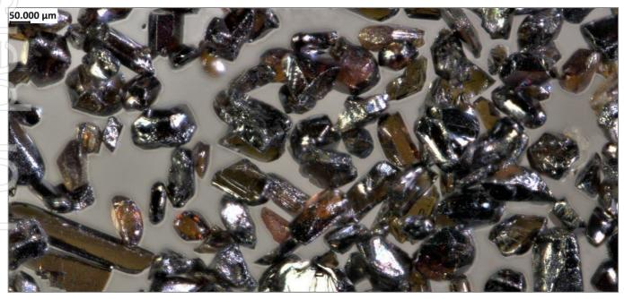
Figure 17: Photomicrograph of high-purity rutile product
