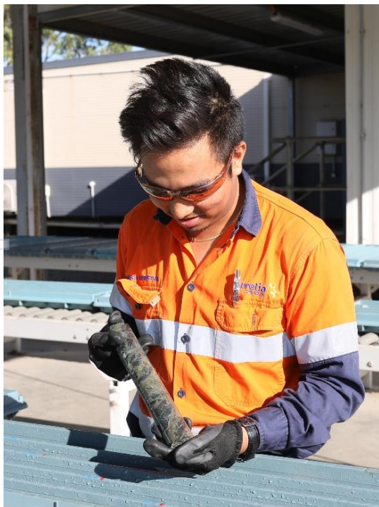
Figure 1: Exploration Geologist, Dinesh Shrestha, examining drill core from Kairos drillhole UD24PK0211 from 291m to 292m grading 6.4% Cu.
