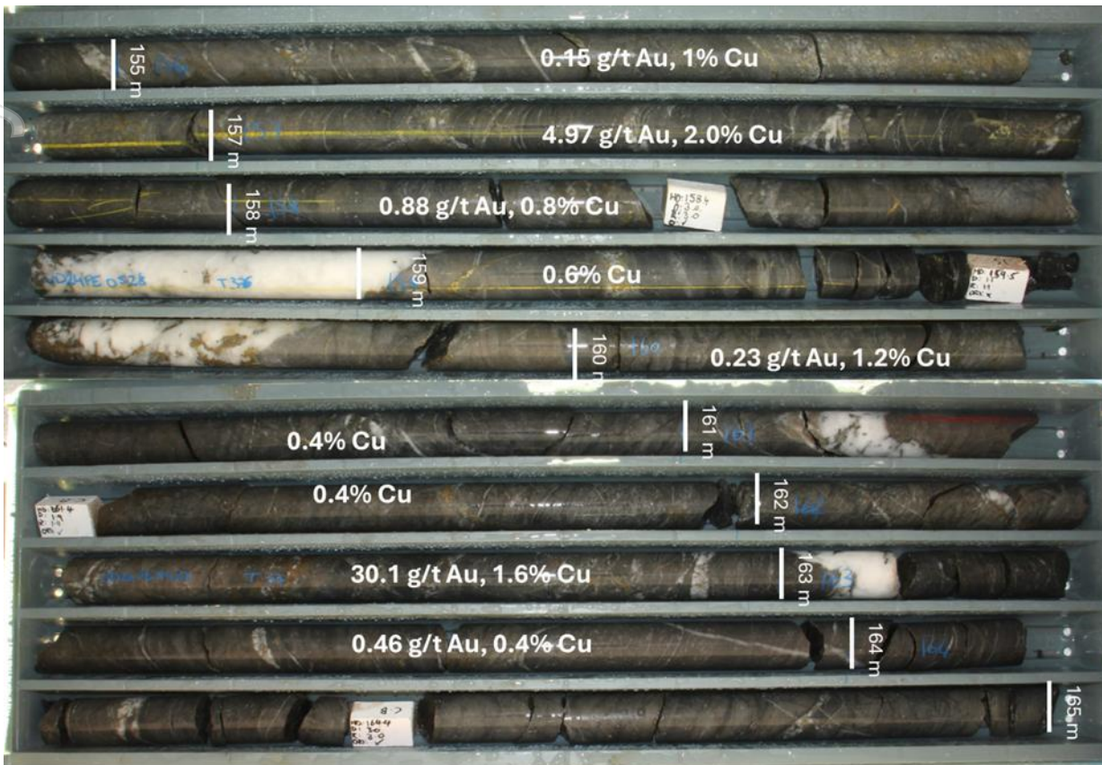
Figure 11: Drill core photo of Hercules drillhole UD24PE0528 highlighting 1.0m at 5.0g/t gold from 156.0m and 1.0m at 30.0g/t Au from 162.0m within 22.9m at 1.6g/t Au from 140.2m.
