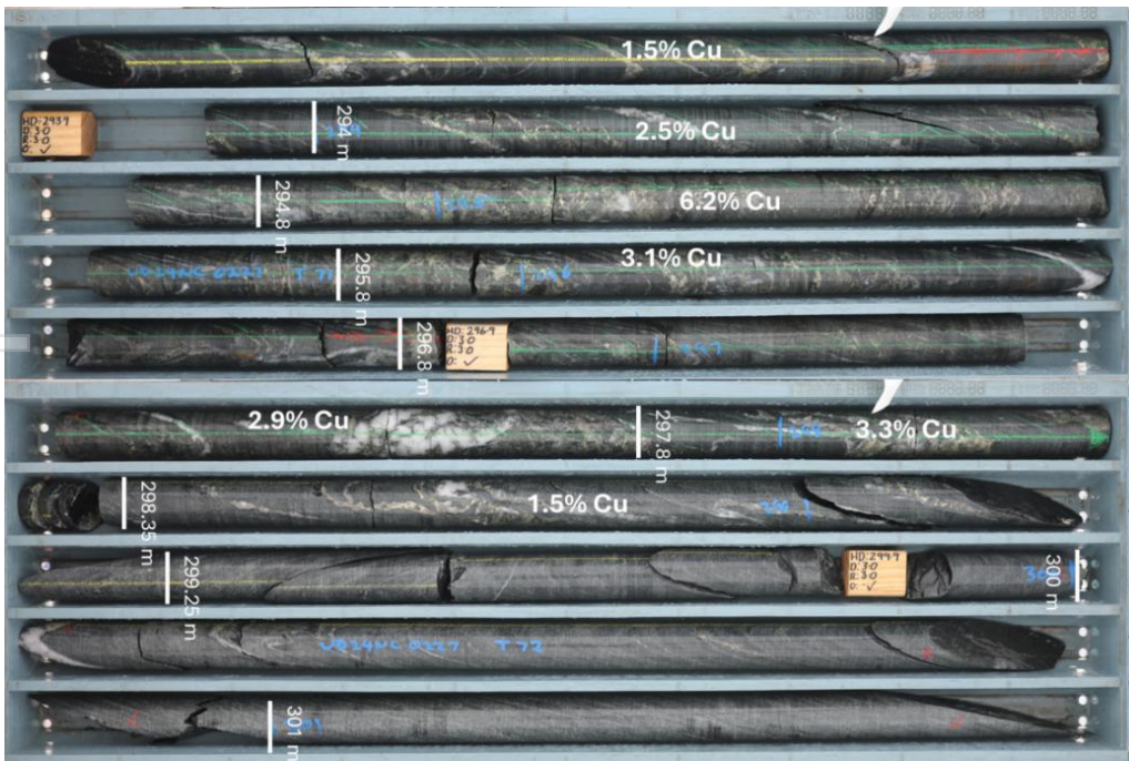
Figure 8: A section of New Cobar drillhole UD24NC0227 highlighting 6.3m at 3.0% copper from 293.0m.
