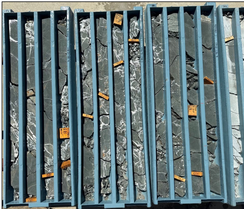
Photo 4. Core tray photo showing brecciated and quartz-carbonate matrix interval from 173.4m to 192m down-hole in SJD001 (½ cut HQ3 drill core).
