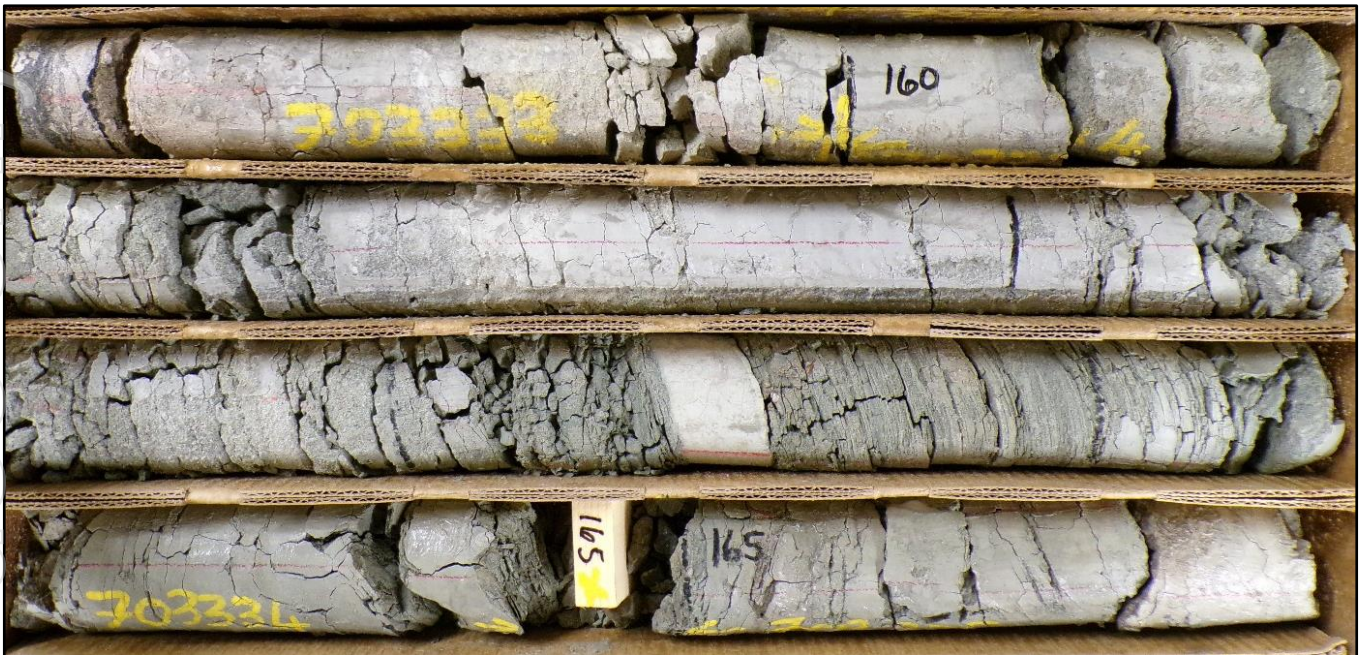
Figure 2. High-grade clay rich RMDD002 drill-core from 48.8-50.3m (160-165ft) which assayed 3,280ppm Li.
