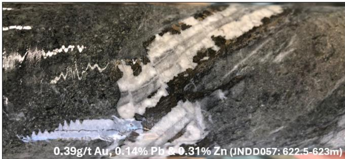
Photo 8. Example of crustiform quartz-carbonate-sulphide veining intersected in JNDD057 at Mitta Mitta.
