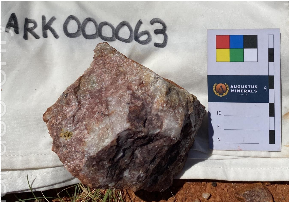
Figure 8 Photo of quartz vein rock chip sample ARK000063 which assayed 30.4g/t Au
