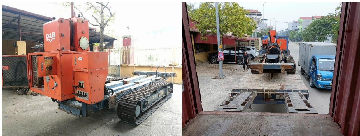
Figure 5: Track carrier and RC sample system from Vietnam being loaded into a sea container for transport to Timor-Leste
