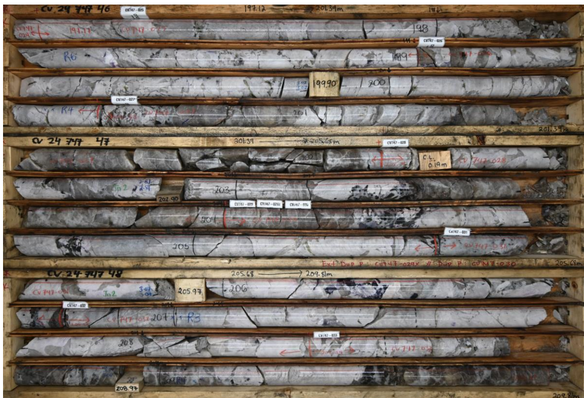
Figure 3: Very large spodumene crystals in high-grade pegmatite from Vega Zone in drill hole CV24-747. Core grades 12.6 m at 4.64% \text{Li}_2\text{O} from 197.2 to 209.8 m, including 4.3 m at 5.55% \text{Li}_2\text{O} .
