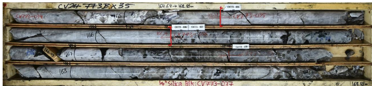
Figure 2: Large spodumene crystal(s) (0.9 m core length) grading 7.11% Li 2 O, the highest-grade drill core sample collected to date at the Property (drill hole CV24-773).
