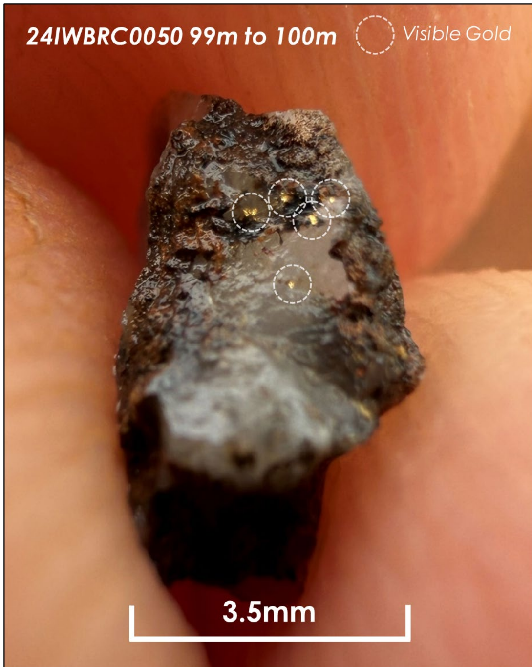
Figure 7: Visible gold evident within and adjacent to an oxidised quartz vein fragment from the 99-100m interval in 24IWBRC0050. The same interval returned an initial 50g fire assay result of 1.7 g/t Au . Additional samples have been submitted for screen-fire analysis.
