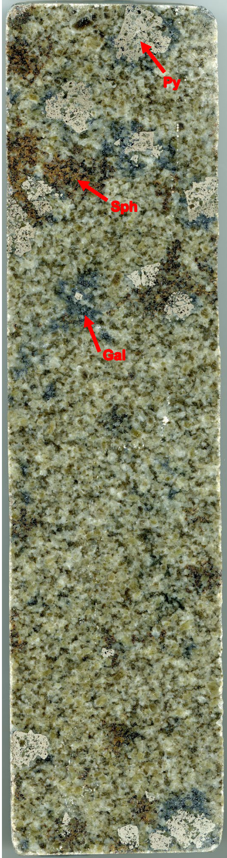
Figure 3: Polished half HQ core from MWDD002 340.25-340.45m displaying pyrite (Py), sphalerite (Sph), and galena (Gal) within a strongly sericite altered albitised leucogranite. This sample is part of a meter section (340-341m) that assayed 9.92g/t Au, 38.7g/t Ag, 0.45% Pb, 2% Zn.
