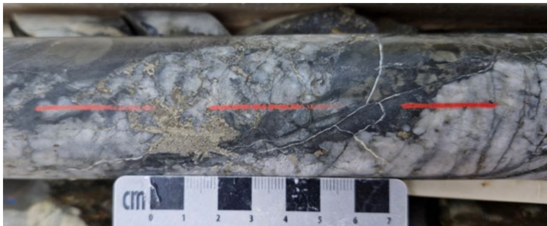
Figure 4: CUTBD03, 145m – Unsampld pyrite(brass-yellow)-pyrrhotite (brown-bronze) in quartz vein (see Appendix 1, Drill Log Summaries and Cautionary Note Page 2).
