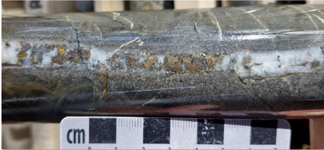
Figure 10: CUTAD01, 225.3m - Unsampled pyrrhotite (brown-bronze)-chalcopyrite (yellow)-pyrite (brass yellow) in quartz vein (see Appendix 1, Drill Log Summaries and Figure 3 Cautionary Note Page 2).
