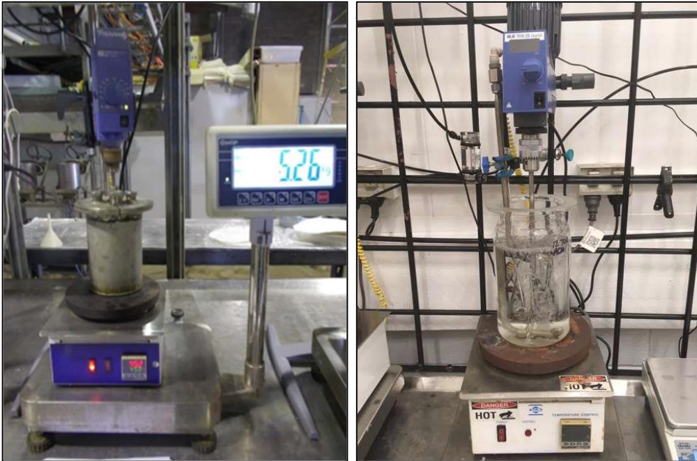
Figure 11. Montezuma Alkaline Sulphide Leaching and Air Oxidation Test Set Up
