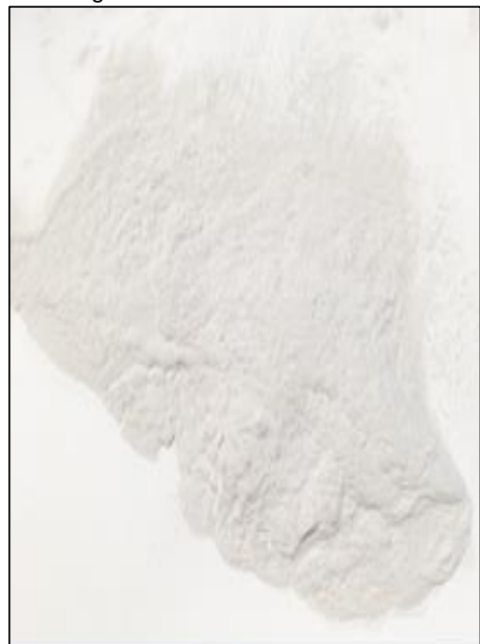
Figure 4. Saleable antimony product sodium pyroantimonate ( \text{Na}_4\text{Sb}_2\text{O}_7 ) produced during metallurgical test work
