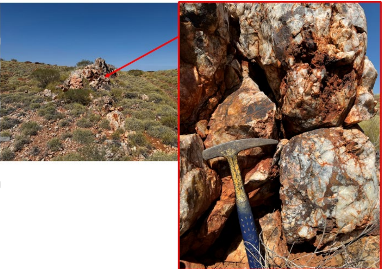
Figure 5. Thorpe Prospect - 5m wide quartz & quartz/iron oxide veining returning 5.9g/t Au & 1% Cu (Sample 24AR22-014)
