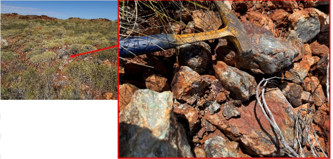
Figure 4. Thorpe Prospect - 3m wide quartz/iron oxide vein returning 45.8g/t Au & 3.7% Cu (sample22AR22-020)
