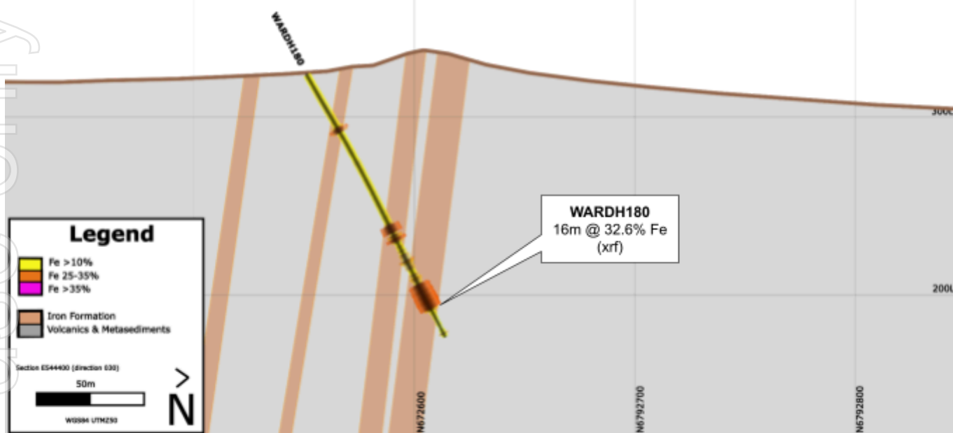
Figure 01: Section through iron mineralisation WARDH00180
