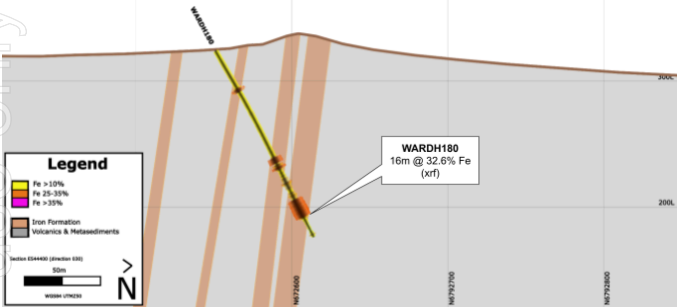
Figure 01: Section through iron mineralisation WARDH00180
