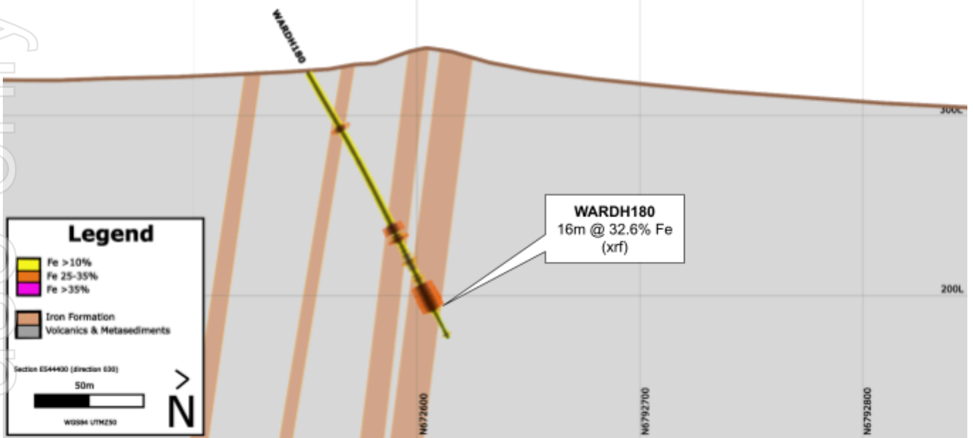
Figure 01: Section through iron mineralisation WARDH00180
