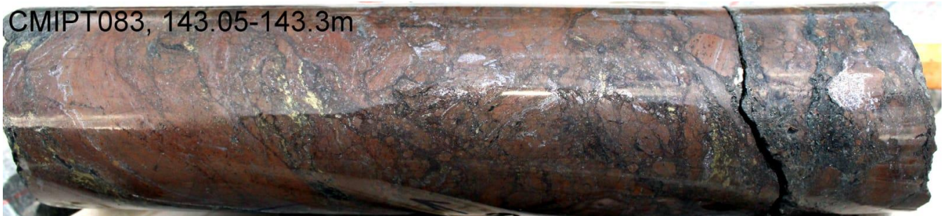
Figure 5. Hole CMIPT083: high-grade massive and brecciated massive sphalerite (red-brown) with lesser galena. Up to 3% chalcopyrite (yellow) is present in places (ASX Release August 6 th 2018).
