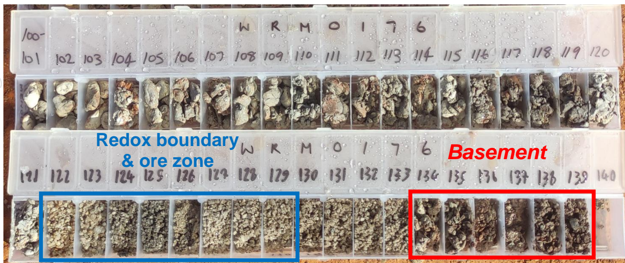
Figure 5: Example of uranium mineralisation within the lower Eyre Formation at Beulah (hole WRM0176).
