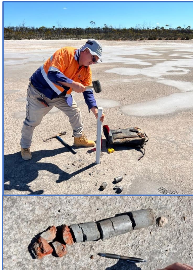
Figure 2. Lake Hope showing the push tube sampling method used to drill out the resource and an example of the lake clay from the push tube showing excellent sample recovery.
