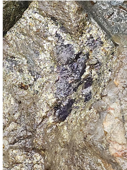
Figure 6 Chalcopyrite rich sulphides at the Chevrier Prospect
