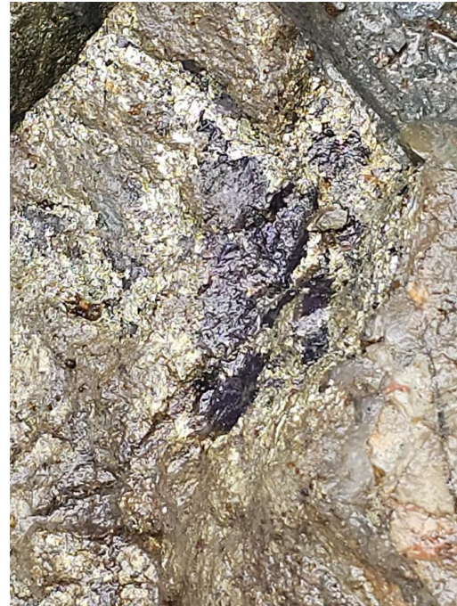
Figure 6 Chalcopyrite rich sulphides at the Chevrier Prospect
