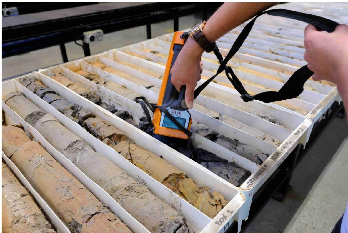
Figure 2: Spectrometer 153 cps Orroroo 2A reduced sediment margin.
