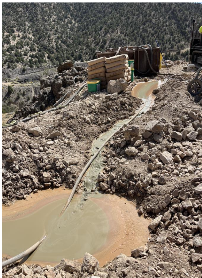
Figure 2: Green copper rich water return during drilling of hole NY2024-DDH2 at New Years.
