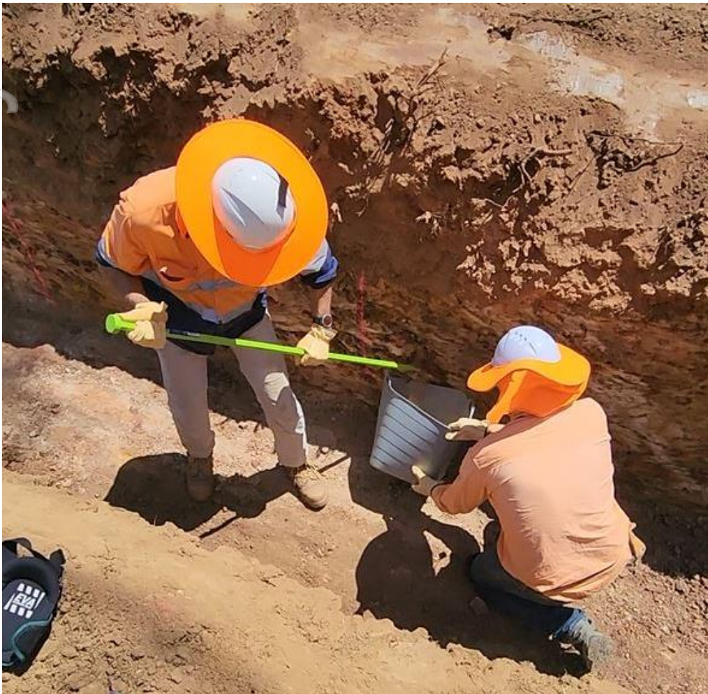
Figure 6: Banshee channel sampling along lower walls of shallow historical trenches
