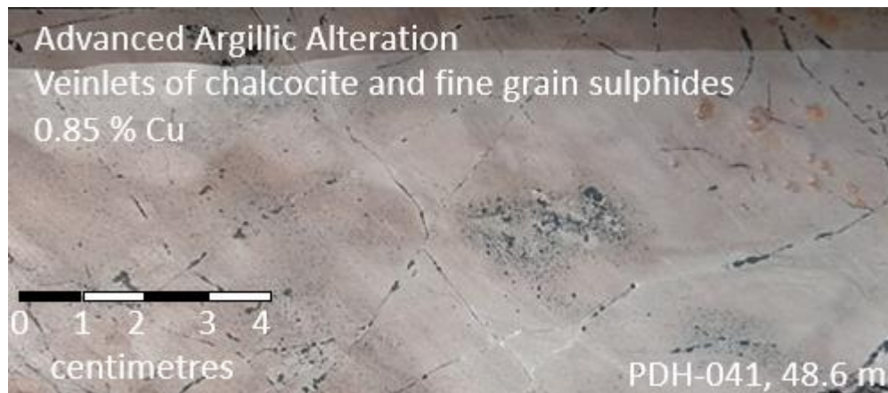
Figure 3-2. Advanced Argillic Alteration, veinlets of chalcocite and fine sulphides. (MA 2024)
