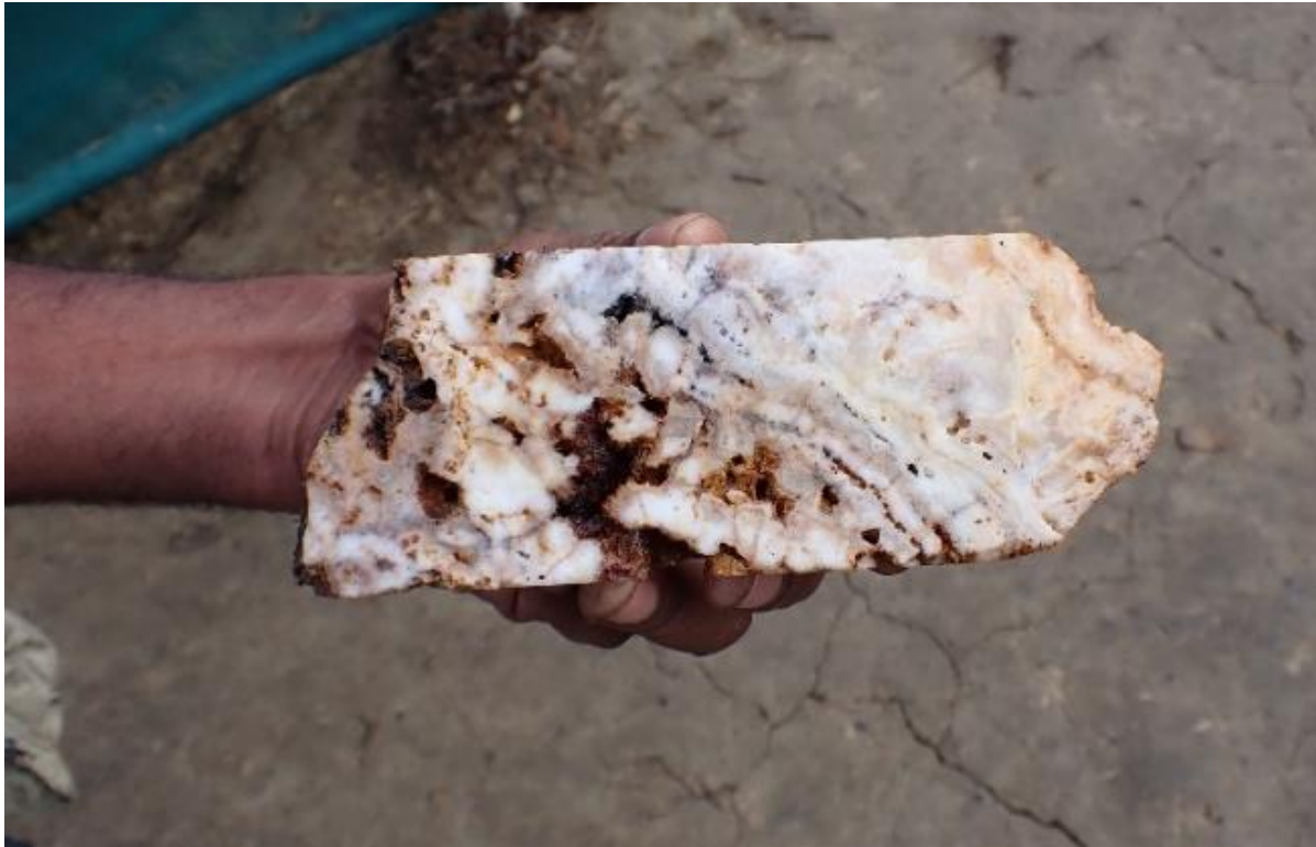
Photo2: Vuggy Colloform Banded Quartz in Taula Vein TDH02 at 23m Depth
