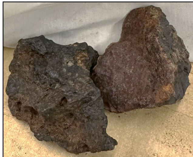
Figure 1: Gossan sample KRP065 rich in iron (24.95%) and manganese (>5%) and exhibiting a vuggy texture.
