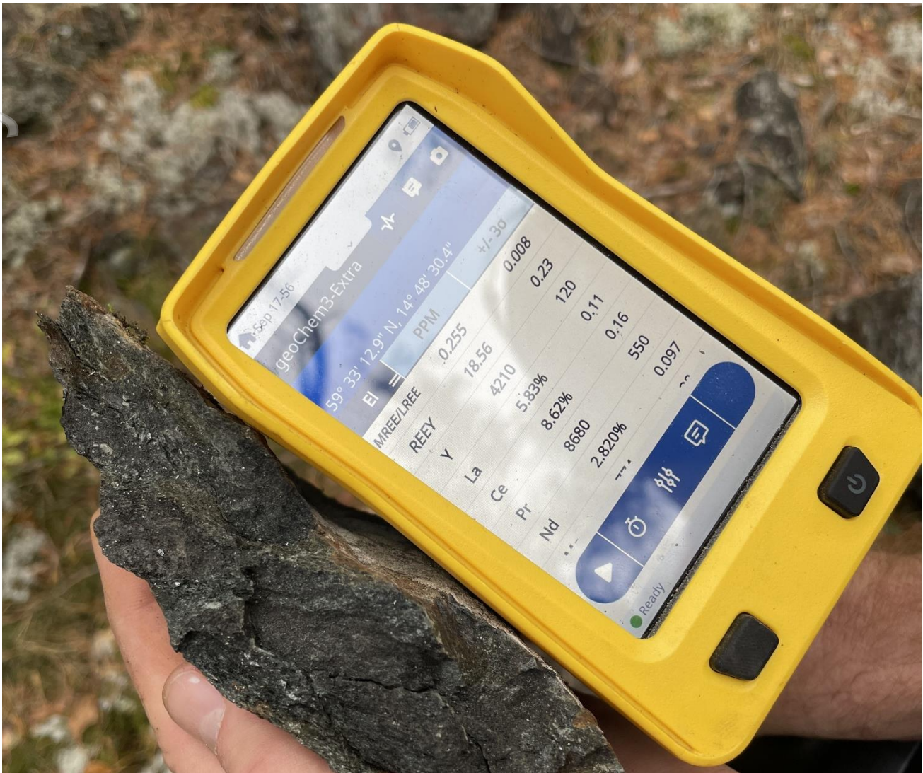
Figure 3: STRR001 sample with pXRF analysis. 489174 East/6601710 North. Sweden SWEREF99 TM reference system and datum. Sample consists of biotite skarn, which is schistose and massive (60% biotite), containing actinolite (15%) and magnetite (up to 5%). Up to 7 cm dull dark brown REE vein/lens (fine grained) along the foliation. REE mineralisation is present in patches or veins concordant with the foliation in the host rock. REE minerals cannot be distinguished specifically. TREE +Y elements are present to 18.56%. pXRF analyses and visual estimates are only indicative and should not be considered equivalent of laboratory analyses. Laboratory assays are expected in late November.
