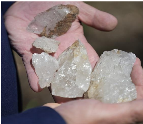
Figure 5: A collection of quartz float samples that show the clarity of the Kingsgate quartz samples.
