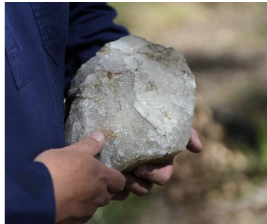
Figure 5: A collection of quartz float samples that show the clarity of the Kingsgate quartz samples.
