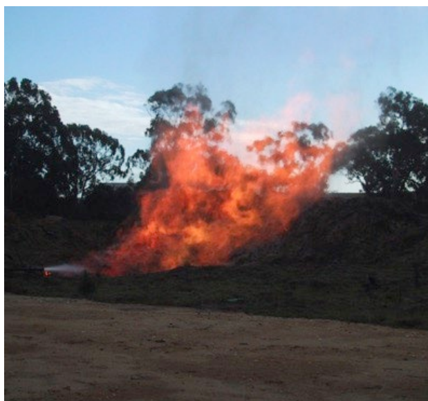
Figure 2: Flaring of Gas at Wombat-1 Gas Well
