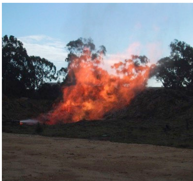
Figure 2: Flaring of Gas at Wombat-1 Gas Well
